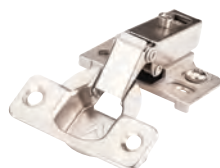
22855-9 1/2" OVERLAY WITH CAM ADJUSTABLE PLATE PRESS-IN 8MM DOWELS
