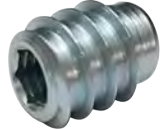
A314 5/16 - 18 X 9/16 ■ ZINC PLATED ■ THREADED INSERT ■ DRILL 14/32" PILOT HOLE
